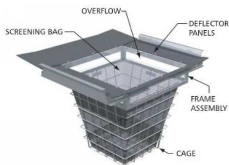
Figure 13: EnviroPod Pit Inlet Trap (Source: Stormwater 360)
